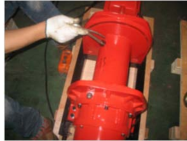
Fig 10 Fixing the wire rope to the drum.
