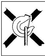
Fig 3 a The sling is applying load to the hook tip
