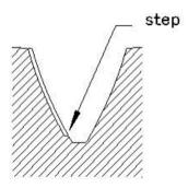
Replace if there is a step on the surface of the gear teeth.
