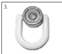
3. Place the house on the bush. The traceability code should be seen.
