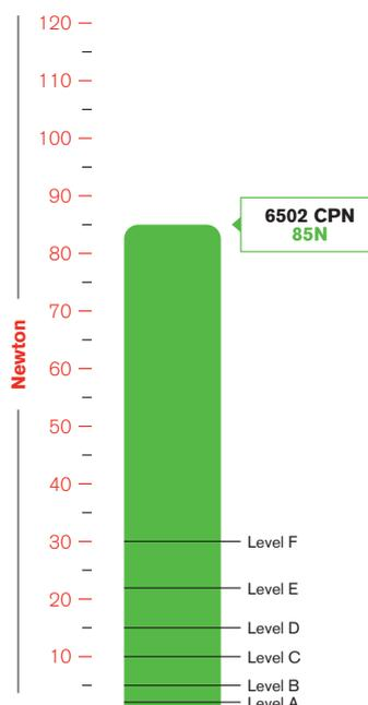
**Needle protection, ASTM F2878**
