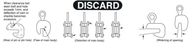
Discard the clamp if obvious flaw or distortion is found in the main body. Defects in the main body can not be repaired in the light of safety. The main body may be cracked or deformed only after several uses if it is used incorrectly. Dent or swelling of main body, or widening of
