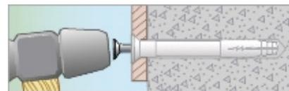
3. Hit the nail with a hammer. For painted 5 mm Nail Plugs use rubber hammer. For dim. 10 mm the plug and nails are supplied separated in the pack. The plug must first be pushed into the hole and then the nail is knocked in.
