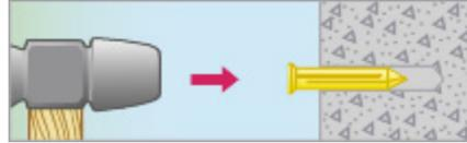
2. Knock the Clips plug into the drill hole. Knock the plug in until it is flush with the surface of the substrate.
