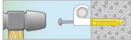
3. Knock in a cable clip with the corresponding nail.
