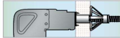
3. Expand using the pliers SAM. When there is resistance and the fixing feels stable the metal expander has reached the correct expansion.
