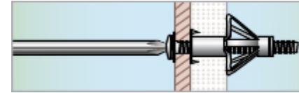
4. Unscrew the screw and secure the detail. The installation is finished.
