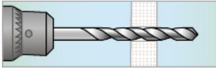
1. Drill the holes. Be careful not to damage the drywall on the back and around the exit hole.
