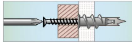
3. Same operation with TF27 with a countersunk head, which can support a detail thickness up to 27 mm.
