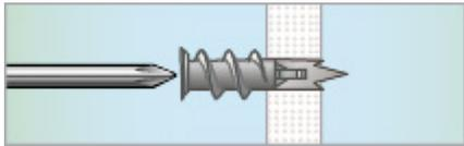
1. Screw the self-drilling fixing directly into the wall. Use a crosshead bits, PZ 2 (Pozidrive) on both the fixing and screw.
