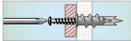
2. Screw on the detail to be secured using appropriate screws. In this example, TP12 with a pan head, which can support a detail thickness up to 12 mm.
