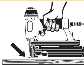
● Lift tool completely from work surface between shots to feed next cap.
