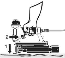
● With a "Dual-Action" trigger, nails can be driven two ways:
